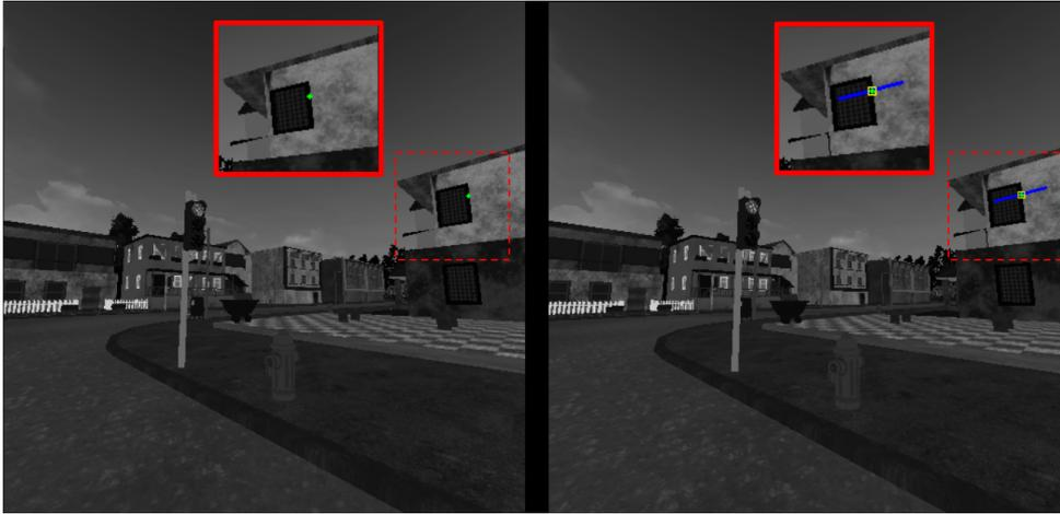
Figure 3: Epipolar line search example with image sequence from carla dataset (left: reference frame, right: current frame). Epipolar line is depicted in blue, matched point is emphasized with yellow border.
