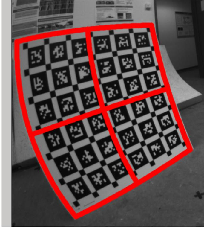
Figure 4.4: One image of a calibration sequence showing the grid region that was taken into account for the calibration. The red lines show the same distortion as the grid itself, verifying correct calibration of the camera parameters.
