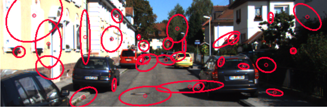
Figure 3.6.: Covariance ellipses for position uncertainties on KITTI seq. 07. The tracks are generated using the Gaussian approximation of the KLT tracking energy function. The PNEC correctly considers the anisotropic inhomogeneous error distributions of the features. For visualization purposes the covariances are sub-sampled and enlarged. Only a sub-image is shown.
