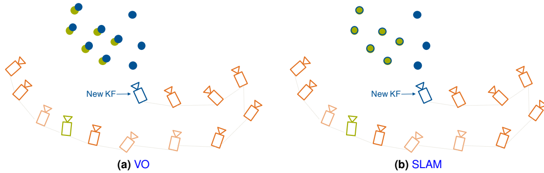
Figure 1.1.: Duplication of map points (which we will also refer to as landmarks) in VO versus their reuse in SLAM systems. In (a), already mapped points hosted in, i.e., relative to, an old keyframe (orange camera) are duplicated when the sensor at the current position (blue camera) revisits the region. Thus, some landmarks (blue) will be mere duplicates of previously mapped landmarks (orange), which is how VO systems typically function. In contrast, SLAM methods attempt to reuse landmark information to better localize the sensor within the map (b), therefore avoiding point duplication.
