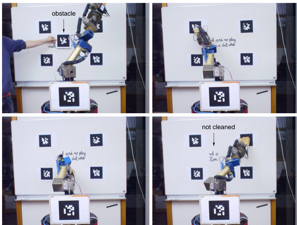
Figure 8.9: During the second reproduction, we introduced an additional obstacle that the robot has to consider using a visual marker. As a result, the robot does not clean the area under the obstacle.
