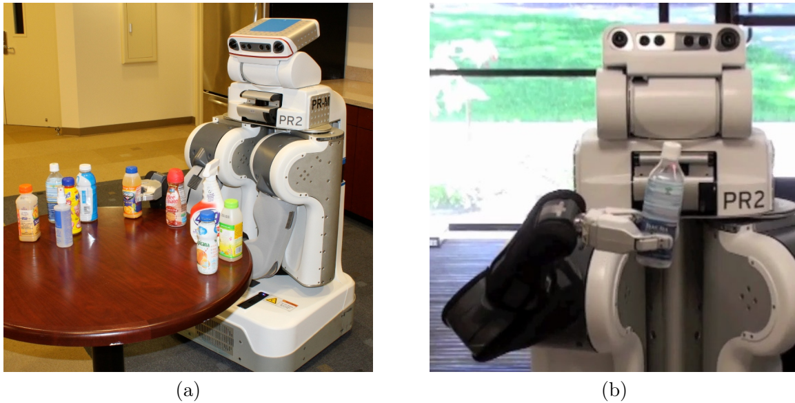
Figure 7.1: (a) To clean the table, the service robot needs to decide which bottles it can dispose because they are empty. (b) The robot detects liquid in a bottle by actuating it.
