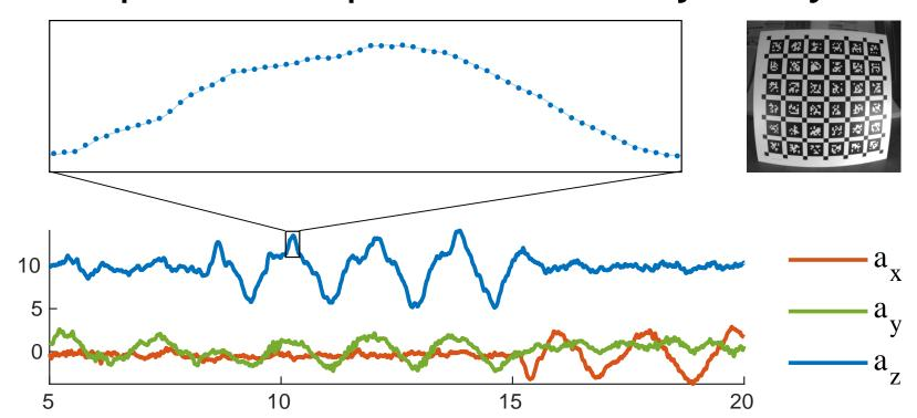
Observations of the calibration pattern are combined with accelerometer and gyroscope measurements to estimate the trajectory and calibration parameters jointly. Accelerometer measurements (dots) are overlaid on the continuous estimate generated from the spline trajectory (line) after optimization.
