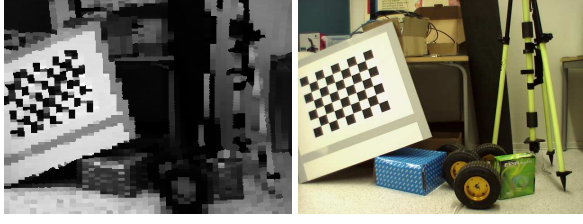
Figure 1: Left: Image intensities plotted with the resolution of the 3D scanner. The laser range readings were projected onto the right image and the closest pixel regions were set to the intensity of the projected pixel for better visualisation. Right: Calibration board used for finding the external parameters of the camera, with a chess board texture and reflective tape (gray border) to locate the board in 3D using the remission / intensity values from the laser scanner.
