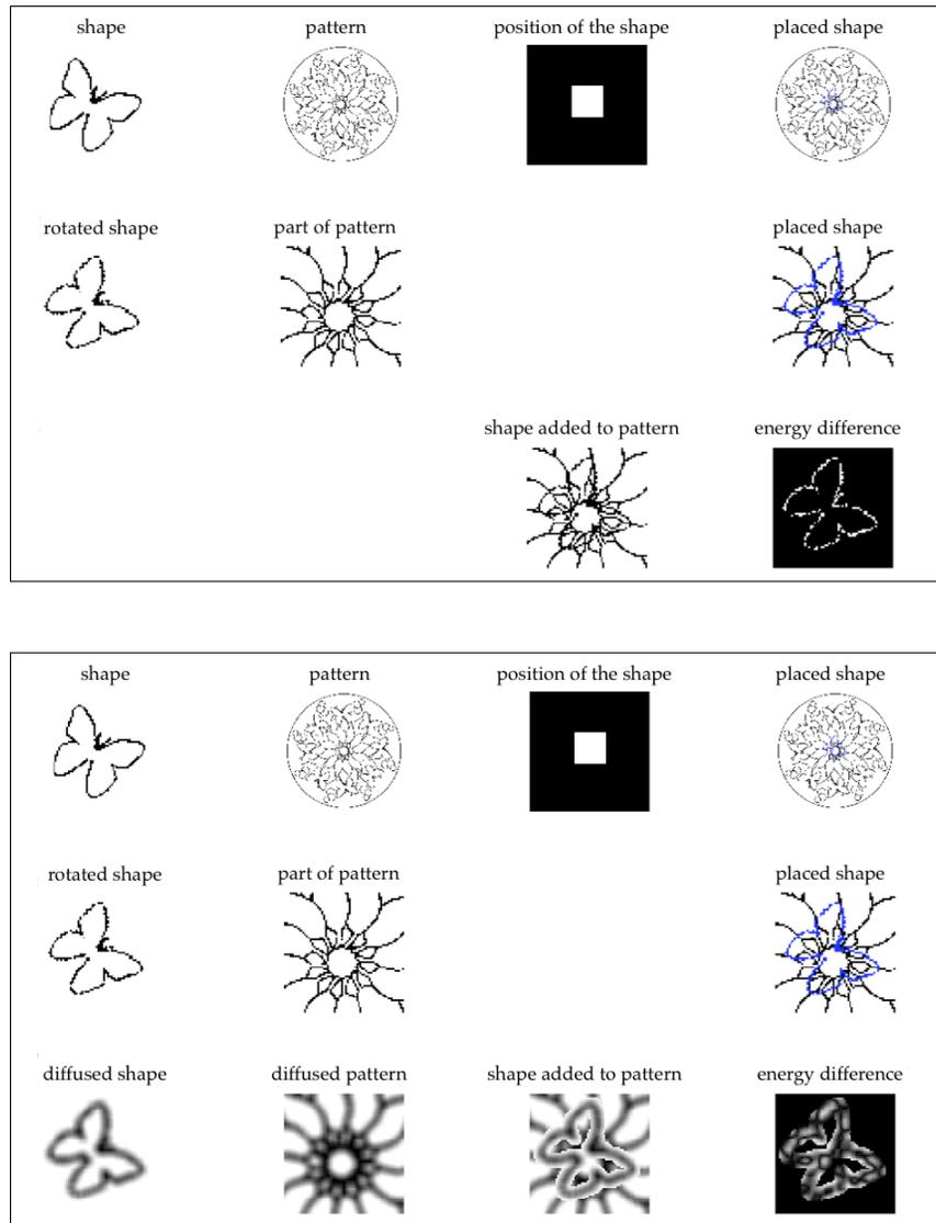
**Fig. 6.** Illustration of cost calculation. When raw binary drawings are used (top), it is hard to tell how well the target figure is located. Observe how matching cost becomes informative when raw binary figures are replaced with diffuse ones (bottom).
