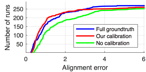
Fig. 9: Comparison of the alignment error for running DSO on sequences for one of the cameras of the TUM Mono VO dataset using either the full ground truth calibration, no photometric calibration or our online calibration.
