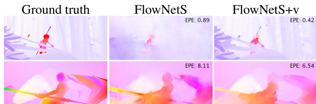
Figure 4. The effect of variational refinement. In case of small motions (first row) the predicted flow is changed dramatically. For larger motions (second row), big errors are not corrected, but the flow field is smoothed, resulting in lower EPE.
