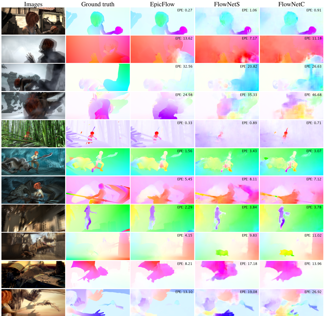
Figure 6. Examples of optical flow prediction on the Sintel dataset. In each row left to right: overlaid image pair, ground truth flow and 3 predictions: EpicFlow, FlowNetS and FlowNetC. Endpoint error is shown for every frame. Note that even though the EPE of FlowNets is usually worse than that of EpicFlow, the networks often better preserve fine details.
