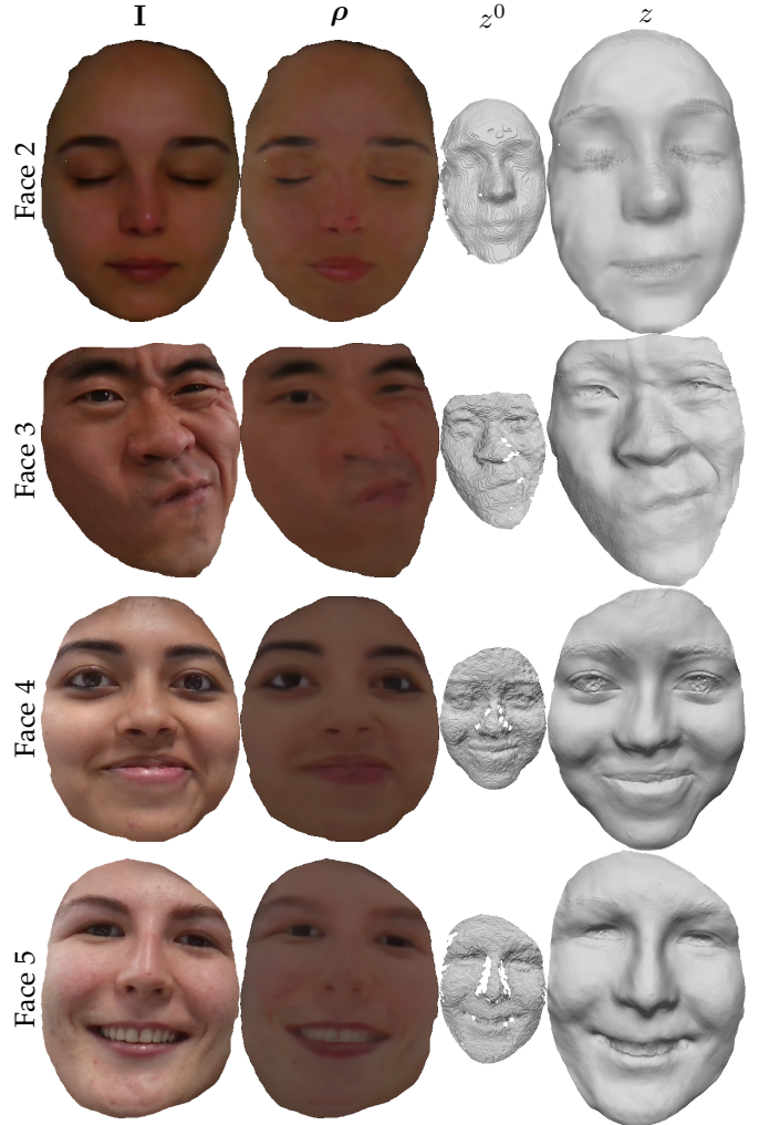
Fig. 5: Results of the proposed variational approach to photometric depth super-resolution, using deep learning to estimate reflectance. Data was captured with an Intel Realsense D415 camera.
