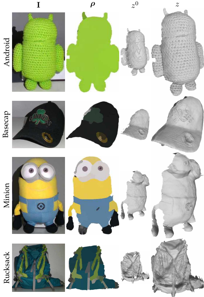
Fig. 2: Results on real-world datasets “Android”, “Basecap”, “Minion” and “Rucksack” we captured with an Intel Realsense D415 camera. All datasets shown here have a scaling factor of 2 between the low-resolution depth z^0 and the high-resolution image I .
