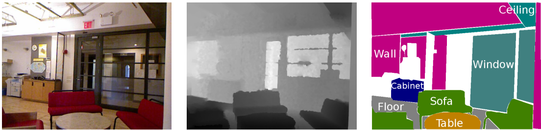
Figure 5.2.: NYU version 1 Depth Benchmark. From left to right: original image, grey level depth map and corresponding ground truth labeling.
