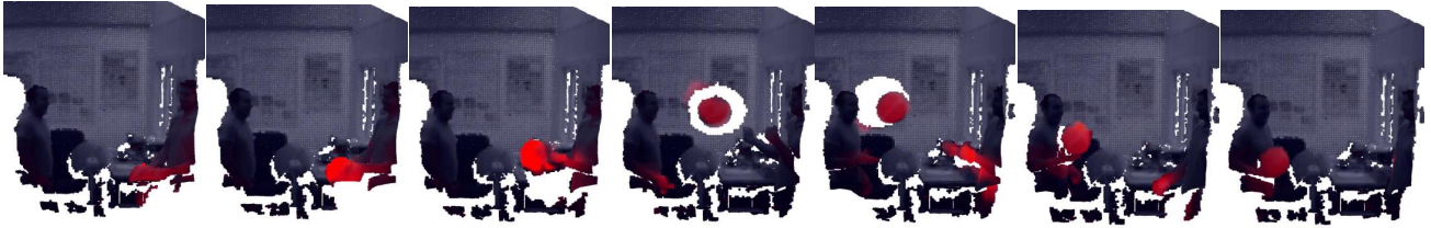
Fig. 4: Temporal sequence of two people throwing and receiving a basketball. The magnitude of the motion field is represented by colors ranging from grey/blue (null velocity) to intense red (fast motion).
