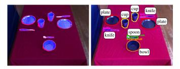
Fig. 7. Segmentation (left) and classification (right) results on the point cloud segments visualized in the Kinect image.
