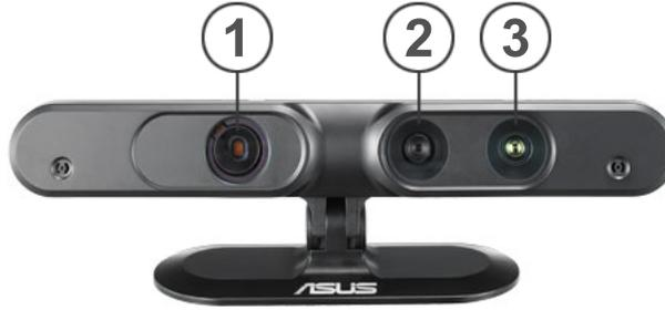
Figure 2.3.: ASUS Xtion PRO LIVE camera: ① IR projector ② RGB camera ③ IR camera [26]
