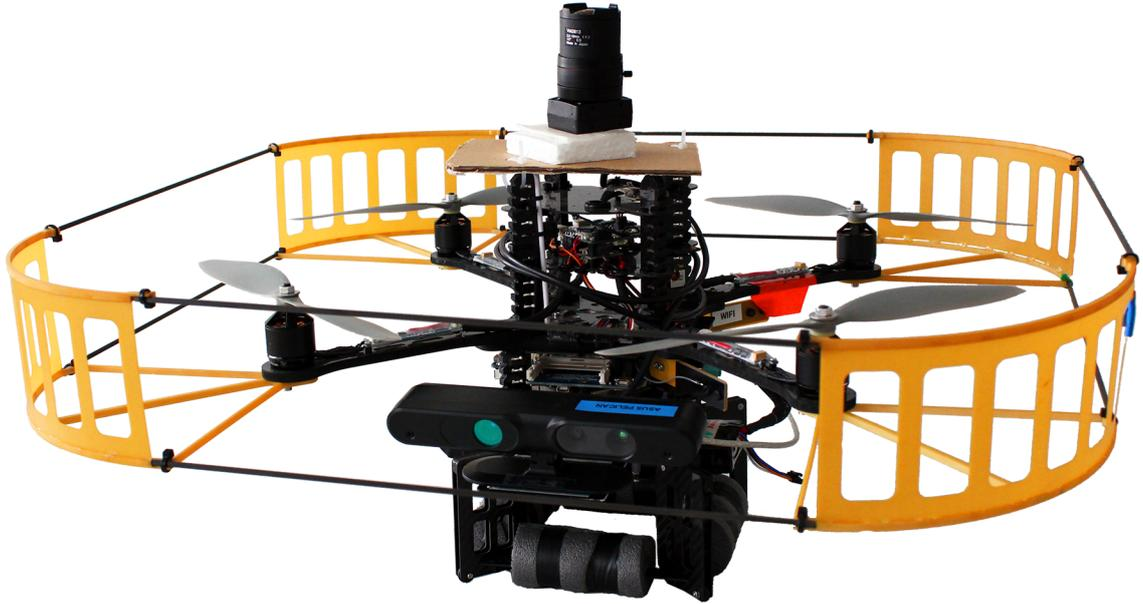
Figure 2.2.: AscTec Pelican quadcopter with payload: the Autopilot Board, the Mastermind Board, a monocular grayscale camera and an ASUS Xtion PRO LIVE RGB-D camera.
