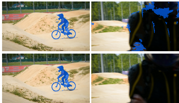
Figure 1: A pixel-classifier trained to predict an object mask ( top row ) performs well when the distribution of object pixels in the training image is similar to the test image ( left ), but often fails if it is dissimilar ( right ). In a transductive inference approach ( bottom row ), we optimize jointly for the test labels and classifier parameters, which successfully prevents the hallucination of object pixels in difficult scenes, such as in the case of occlusion ( right ), cf. Section 4.2.
