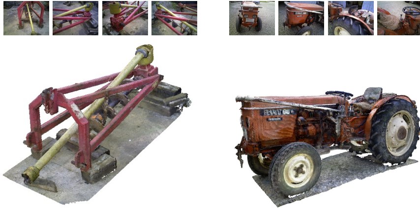
Fig. 5: Left: 3D reconstruction of a soil auger, reconstructed from 2349 RGB-D frames. Right: 3D model of a tractor, reconstructed from 2087 RGB-D frames.
