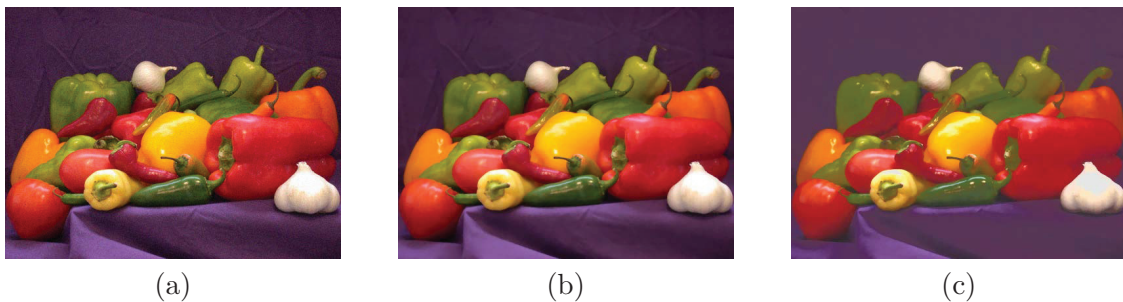
Figure 6. Example of incorporating a nonconvex tonemapping term into the ROF model. (a) Noisy image with small range of values. (b) TV denoised image. (c) Image after TV denoising along with encouraging intensity values to be either 0 or 1.
