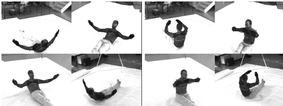
Figure 30: Example images of a Tracked sit-up sequence. During the sequence, parts of the arms occlude with the torso. The back bone joint is crucial for a successful tracking of the sequence.
