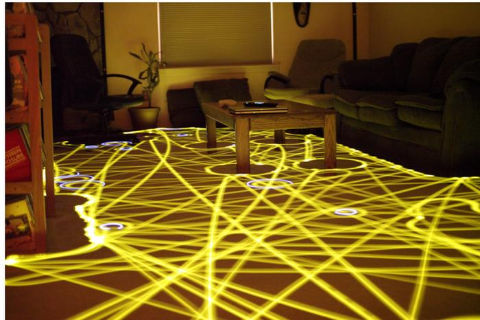
**Figure 1.2.** A time-lapse image of the Roomba [44] as it moves around a room. Odometry helps prevent cleaning the same positions repeatedly.
