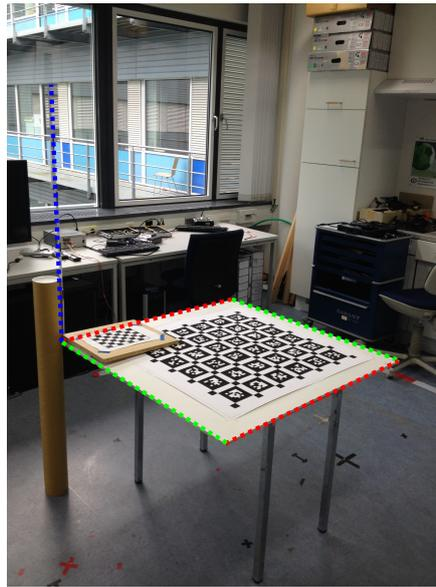
**Figure 8.6.** The setup for the scale experiment. The center board is one meter square and the vertical measuring stick is one meter tall.
