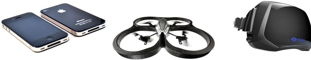
Figure 4.1. The iPhone 4S, AR Drone, and Oculus Rift all contain low cost MEMS IMUs.
