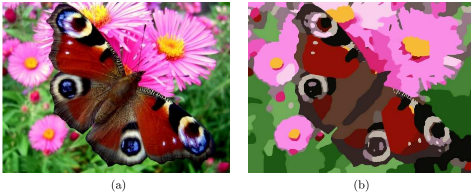
Figure 1.8: An example of a piecewise constant approximation using the MS model (a) the original image f (b) the piecewise constant function u with 15 regions. These images are taken from [2].
