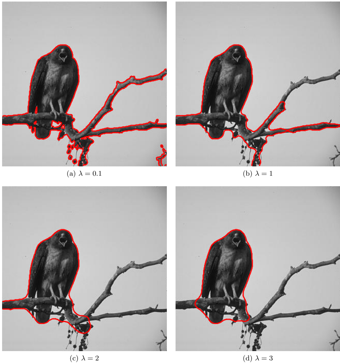
Figure 4.9: Segmentation results for different values for \lambda . With increasing \lambda the perimeter of the contour is stronger penalized, leaving out elongated structures i.e. the branches in the above scene. This image is taken from [45].
