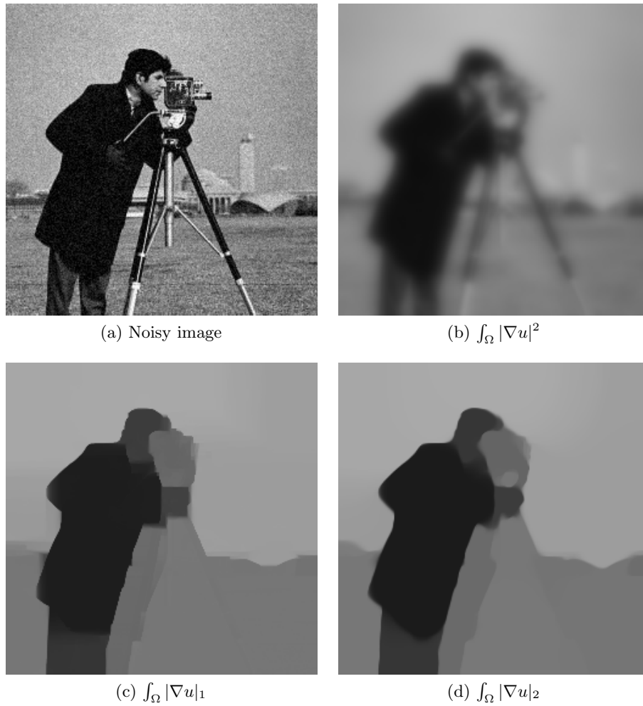
Figure 1.1: Comparison of 3 regularizations of the noisy image (a). Image (b) is a result of a quadratic penalty. Image (c) results from an anisotropic regularization. Image (d) is isotropically regularized.
