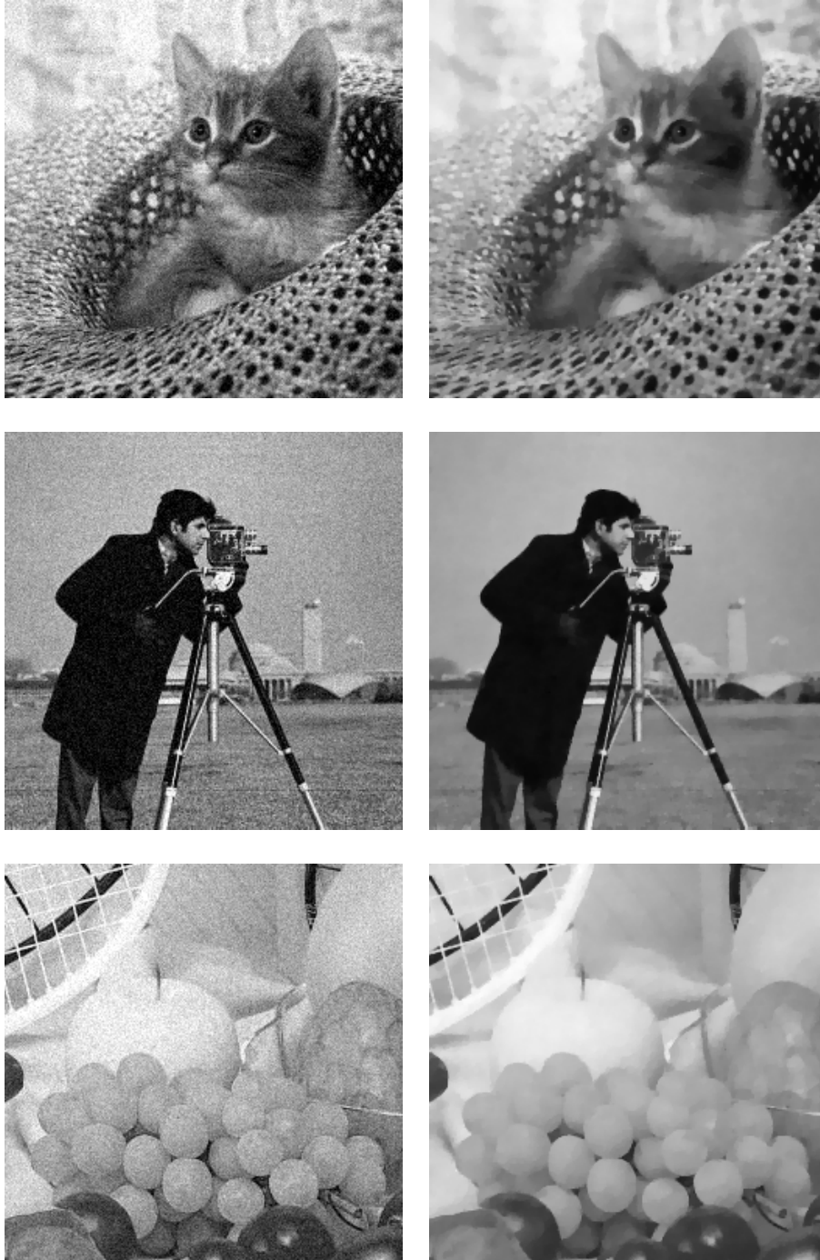
Figure 4.3: The denoising results with the PDAS algorithm for \lambda = 15 .
