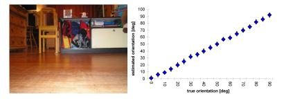
Fig. 5. Experiment conducted in a ordinary, but brightly lit living room at a private home. The robot was rotated manually in steps of 5°. The robot's heading estimates have been plotted against the true orientation.
