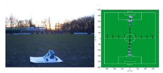
Fig. 7. Experiment conducted at the Zeeburgia outdoor soccer field in Watergraafsmeer, Amsterdam. The robot was moved across the whole field on its primary axes. The arrows display the reported heading, while the blue arcs around the arrow visualize the reported variance. The heading estimates point nicely in direction of the opponent goal.
