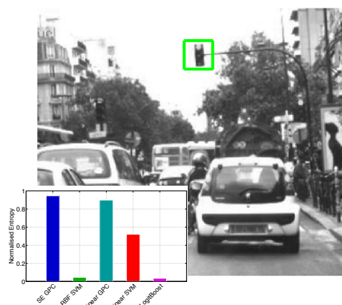
Fig. 1: Uncertainty in classification output as measured using normalised entropy for traffic light detectors based on five different classification frameworks applied to the window shown in green. Note that all classifiers incorrectly label this window as background (class decisions are not shown). However, the GPC variants do so with a significant amount of uncertainty while the others are inappropriately overconfident. Mission-critical decisions based on overconfident output will lead to catastrophic failure while an appropriately high amount of uncertainty when committing a mistake allows for remedial action to be taken. Providing this more germane output is the introspective quality we seek.
