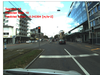
Fig. 1. Example of a traffic light scenario (label 10) detected by our algorithm. The suggested action is a braking maneuver.
