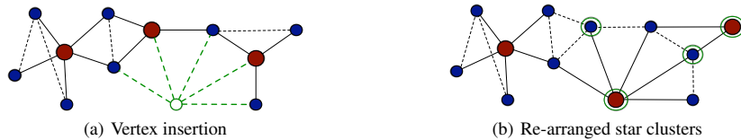
Figure 4: (a) A new data point may introduce additional links in the similarity graph (green) affecting adjacency and hence the validity of the current minimal star cover. (b) Inconsistent stars are re-arranged (green circles). The number of broken stars largely determine the running time. On real graphs, the avg. number of stars broken is usually small (experimentally verified) yielding an efficient incremental approach.
