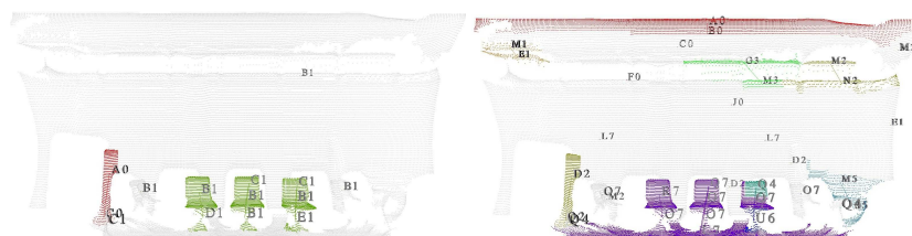
Fig. 7: The results of object discovery with (left) and without (right) saliency computation. All connected segments are considered objects for categorization. Objects are colored by their local class label.
