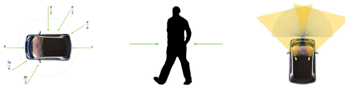
Fig. 2 Left: For car classification, we use codebooks from 7 different views. For training, mirrored images are included for each view to obtain a wider coverage. Center: For pedestrians we use 2 codebooks of side views with mirroring. Lateral views have sufficient information to generalize frontal/back views. Right: Setup used for the city data set. Only a small overlap of the cameras' field of view is used to cover a larger part of the laser scans. No stereo vision is used in this work.
