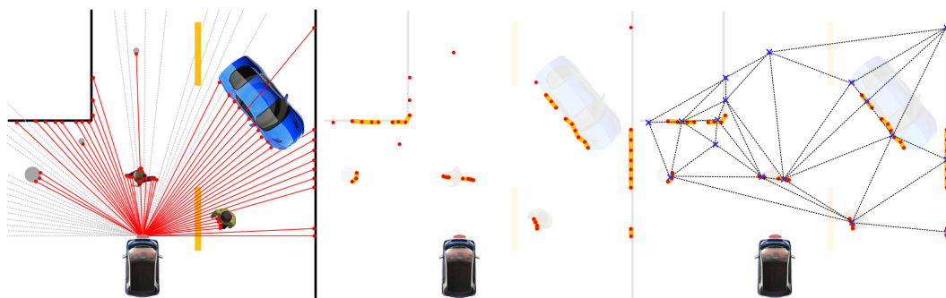
Figure 3.2.: An urban environment with cars, pedestrian and other objects as it is perceived by a 2D laser. Left: Laser beams are shown in red, circles represents the measured points. Gray beams indicate out of range data due to material reflections, sun related effects and particular object poses. Center: Resulting Jump-Distance Clustering of the scene. Orange lines depicts consecutive points segmented in the same cluster. Right: A Delaunay triangulation is computed on the centroids of the segments. This defines graph structure used for the CRF.
