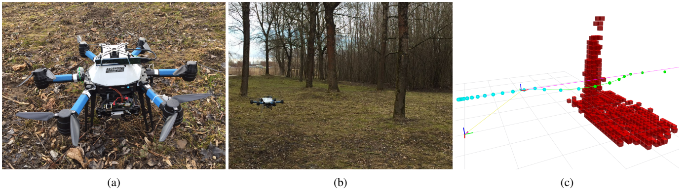
Fig. 4: Real world experiment performed in the outdoor environment. The drone (AscTec Neo) equipped with RGB-D camera (Intel Realsense R200) is shown in (a). In the experiment, the global path is set to a straight line with goal position 30 meters ahead of the drone and trees act as unmapped obstacles that the drone has to avoid. Side view of the scene is shown in (b) and visualization with planned trajectory is shown in (c).
