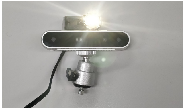
Figure 5: Our setup we used to capture real-world data. An LED light source is attached to an Intel RealSense D415 RGB-D camera. We then move the camera to capture the objects of interest, see Figure 6. Different illumination is induced by camera motion and the attached LED.
