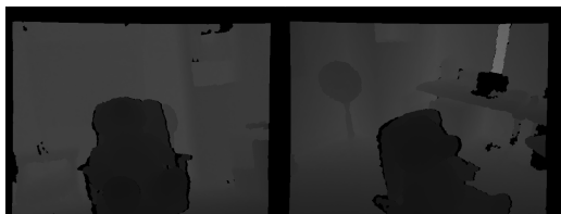
Figure: A couple of depth maps which gives the distance between the camera and the surface
