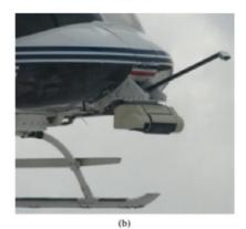
Fig. 1: (a) Landing pad used during experimentation (b) Sensor head mounted on the nose of the helicopter carries
