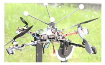
Fig. 1: A picture of the prototype on a testing gimbal
