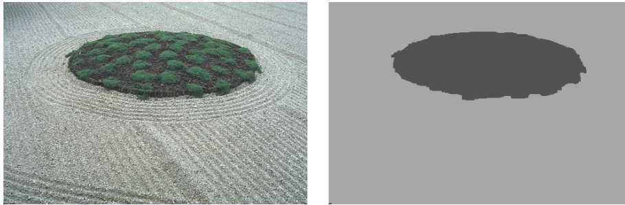
Figure 1: The figure shows the input image and a global minimizer of (5) for parameters \lambda_1 = \lambda_2 = 0.0001 , \mu = 1 , \nu = 0.1 . The optimal foreground and background colors were found as c_f^* = 81 and c_b^* = 167 .
