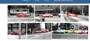
Yellow: global minimum of E; Blue: feature-based car detector; Red: global minimum of the combination of E with detection results (detection is included as a constant potential)
