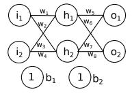
$C = \sum_{i=1}^{2} (t_i - a_i)^2$  where  $t_i$  is the target value for the respective output neuron  $o_i$  and  $a_i$  is the output of the neuron  $o_i$ . Input/output of  $h_1, h_2, o_1, o_2$  is computed as  $z_i^l = \sum_j w_j \cdot a_j + b_l$ ,  $a_i^l = \sigma(z_i^l)$  where  $\sigma(\cdot)$  is any activation function.
