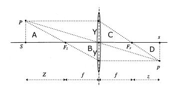
The above drawing shows the perspective projection of a point P (observed through a thin lens) to its image p.
