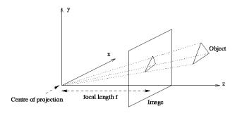
To simplify equations, one flips the signs of *x*- and *y*-axes, which amounts to considering the image plane to be in front of the center of projection (rather than behind it). The perspective transformation  $\pi$  is therefore given by
