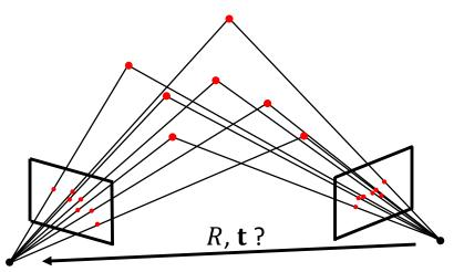
Determine relative camera pose (*R*, **t**) from keypoint matches
