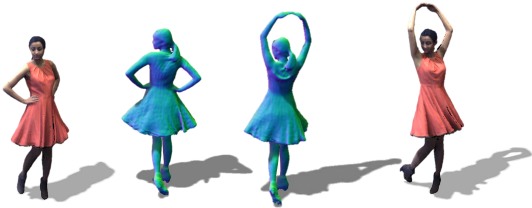
Figure 2: Real-time reconstruction of a challenging scene using the Fusion4D pipeline. Fine details like the hair and dress of the performer are reconstructed faithfully. Furthermore, the large topology change caused by the performer moving her hands does not break the reconstruction.
