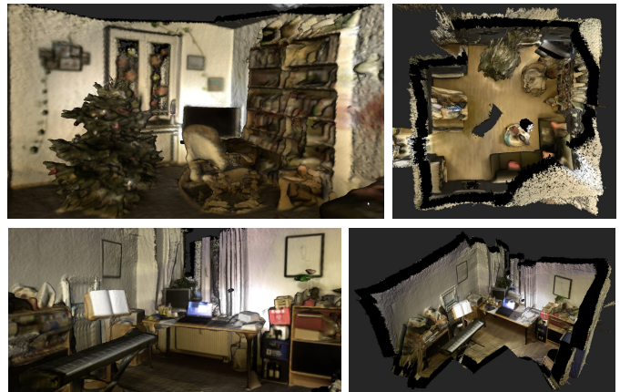
Fig. 1: Reconstruction of a room with a handheld sensor using our approach. Camera tracking and reconstruction runs in real-time on a laptop and provides live feedback to the user. Top row: living room. Bottom row: study room.
