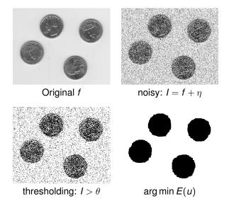
Minimization of the discrete two-region model using graph cuts
