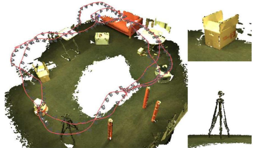
Figure 1. Scene from our benchmark reconstructed in real-time with ca. 335'000 surfels, with keyframes and estimated trajectory.
