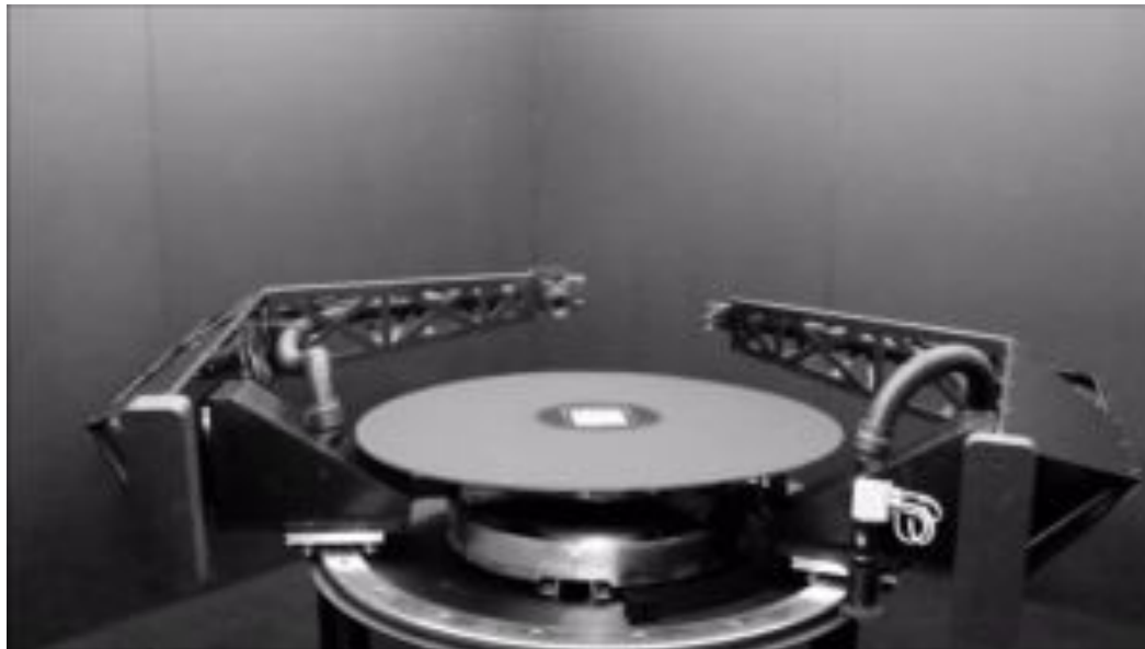
Figure 9. Gonioreflectometer, by Robotae, 2017, retrieved from https://www.youtube.com/watch?v=LsfkAbUUXZU
