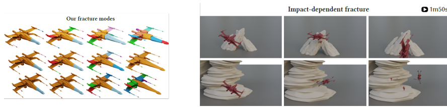
Figure 7: The prefractured modes once evaluated can be used to simulate different impacts from [Sellan et al. 2022]
