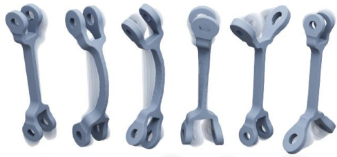
Vibration modes = a shape's natural deformation patterns
