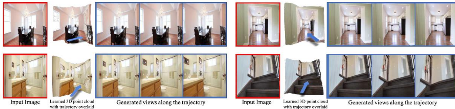
Figure 1: End-to-end view synthesis. Given a single RGB image (red), SynSin generates images of the scene at new viewpoints (blue). SynSin predicts a 3D point cloud, which is projected onto new views using our differentiable renderer; the rendered point cloud is passed to a GAN to synthesise the output image. SynSin is trained end-to-end, without 3D supervision.
